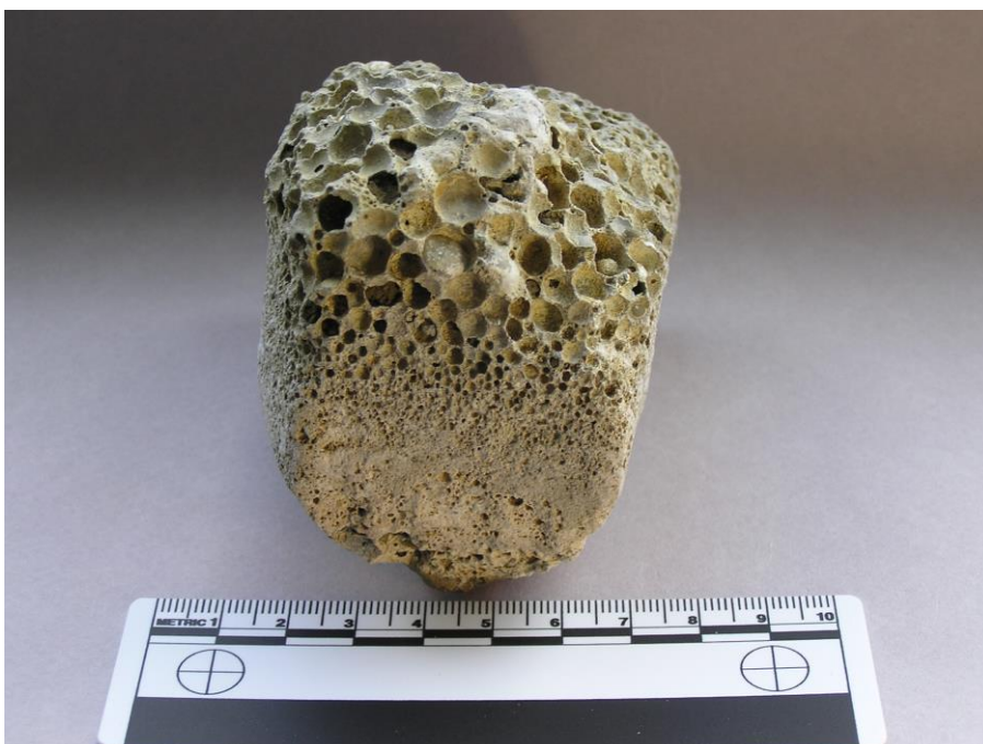
Photograph 3. View of a piece of slag-like material, showing the variable size of the gas vesicles.
