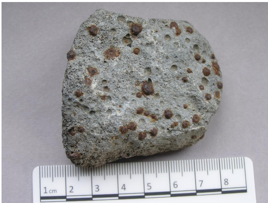
Photograph 4. View of a piece of slag-like material containing spherules of an iron-rich material.
